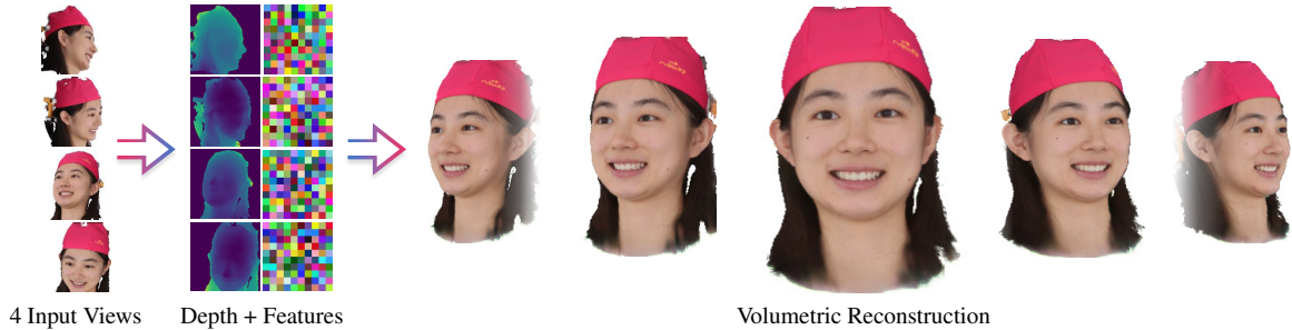
Figure 1. Based on sparse input views, we predict depth and feature maps to infer a volumetric scene representation in terms of a radiance field which enables novel viewpoint synthesis. The depth information allows us to use input views with high relative distance such that the scene can be captured more completely and with higher synthesis quality compared to previous state-of-the-art methods.
